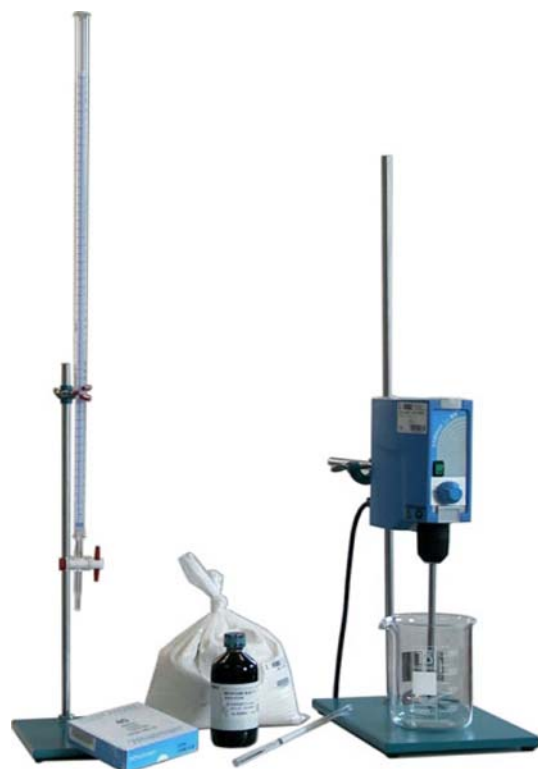
Fig. 3 Methylene blue test equipment
