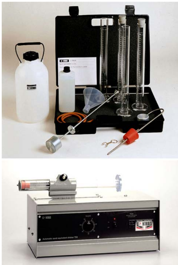
Fig. 2 Sand equivalent test equipment
